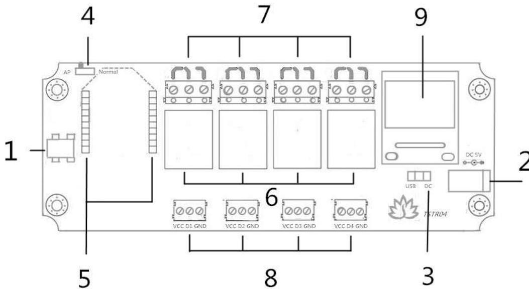
1. Mini USB Port: this port is used to communicate between TSTR04 and computer when you choose the USB mode to control your board, meanwhile, computer can power TSTR04.
