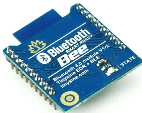
Plug Bluetooth Bee V2 module to TSTR04, make sure set the configure switch to “Normal” position. Here we use remote control, so set the power jumper to DC power mode, and power the board by DC 5V power.
