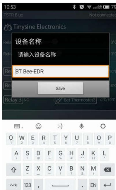
(5) In this step you need to input pair code, the default pair code is **1234**. When your phone has connected to TSTR04, the interface will show “**connected: BT Bee-E**” at the top.
