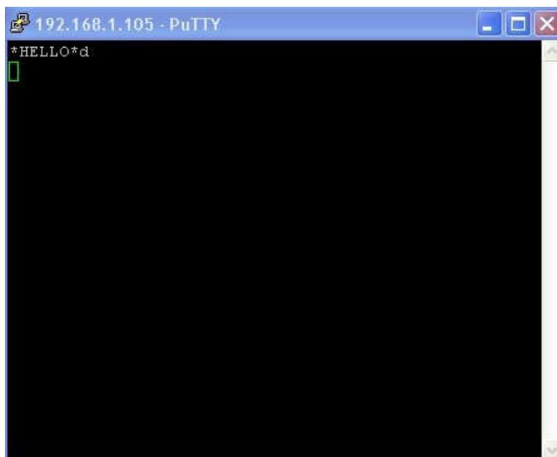
Send ASCII command 'd' ->All relays on
