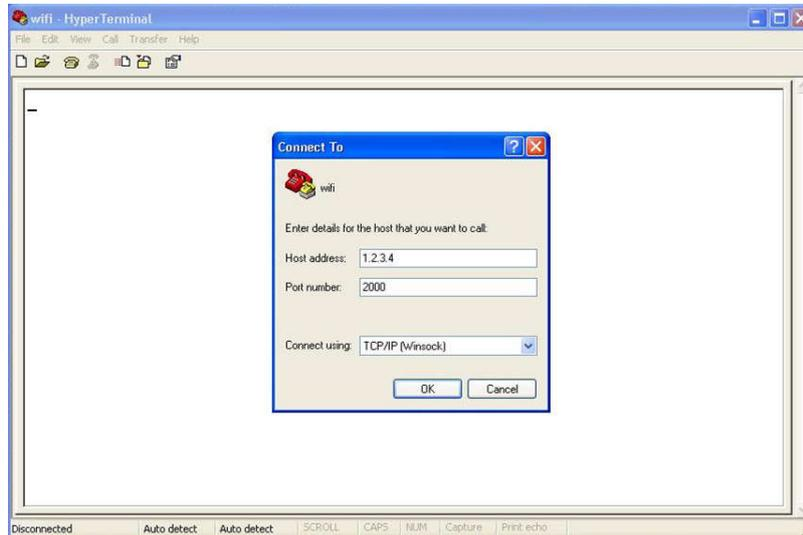
(5) Once connected with a proper IP address, you should see the response **\*HELLO\***. Input escape sequence **\$\$\$** to make the WiFiBee enter commands mode, and Hyper Terminal should return **CMD** to you.
