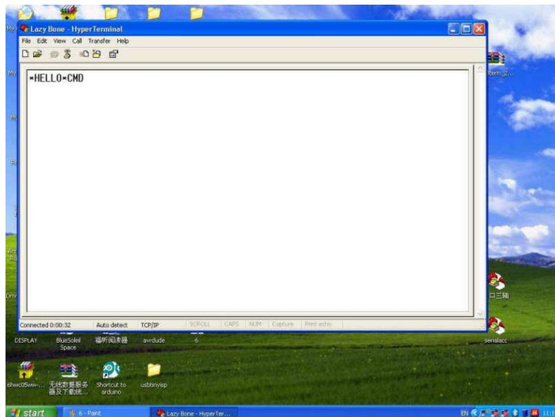
(6) Now you can setup the WiFiBee's settings. Input every command on your keyboard, and click the **Enter** button after each command to send. The Hyper Terminal should return **AOK**.
